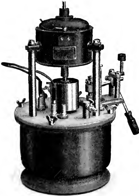
FIG. 189.—Mercury interrupter with gas di-electric. (Schall.)
